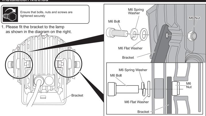
2. Loosen the M6 Bolt on either side of the lamp, Then adjust the vertical angle to suit the installation orientation and available space. After adjustment, ensure the bolts are tightened securely to prevent the lamp from tilting due to vibration.
